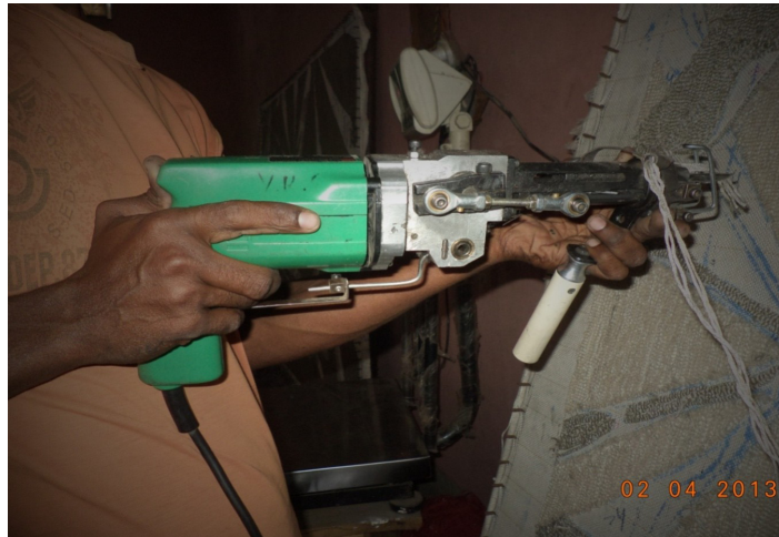
Figure 7: Artisan weaving the carpet with tufted guns
