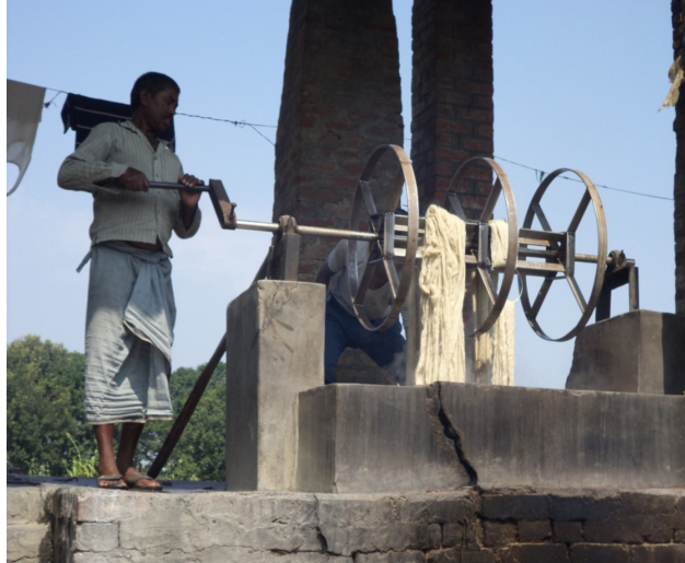
Figure 1: Manual dyeing process in traditional kuda
